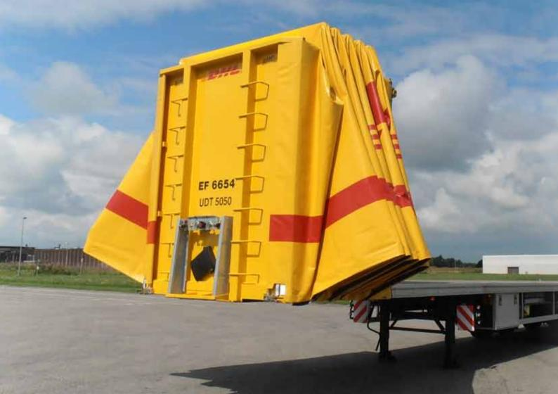
The Netcap LPS sliding tarp systems, which completely cover the platform of a truck or trailer within seconds, are used by operators worldwide to transport steel profiles, coils, wood, glass, containers, machines, automobiles etc, are very stable while being light weight and easy to operate by a single person.
